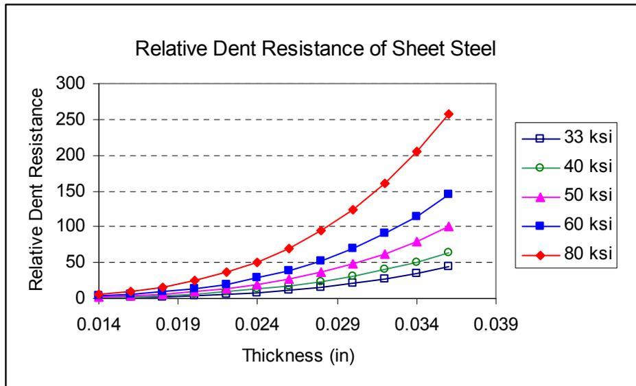
Figure 1. Relative dent resistance of sheet steel.
