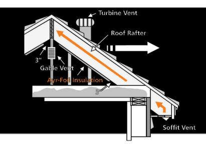
In the summer, most of the heat entering homes and buildings comes through the roof. Using a reflective foil like AYR-FOIL™ aluminium-aluminium or aluminium-kraft paper saves on air conditioning costs and maintains a comfortable temperature inside. AYR-FOIL™ attic barrier can reduce heat gains through the attic by as much as 78%. Both products available are perforated to eliminate condensation problems. AYR-FOIL™ radiant barriers can also improve fibrous insulation performance in the winter.
